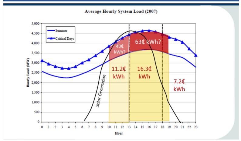
So if the high value electricity is in the late afternoon, it would make sense to face the array to the SW to reduce your air conditioning load.
